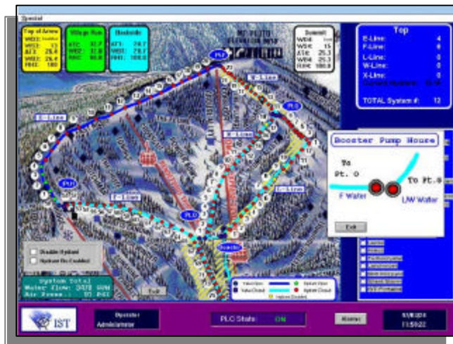
Mountain operation screen for snowmaking
